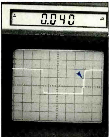
Figure 5. The clock signals must have the correct frequency and amplitude, and they must be free from glitches. This glitch causes the microprocessor to act as though it is defective.
